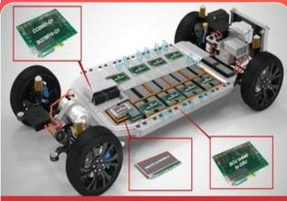
Battery Management Systems (BMS) are the silent drivers behind electric vehicle performance, safety, and efficiency.
